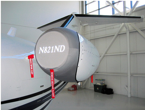
Citation Mustang Intake/Exhaust Cover, "Bikini" Type and leading edge Pylon inlet plugs
