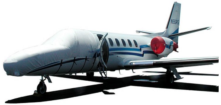
Cessna Citation Nose/Cockpit Cover, Engine Covers
