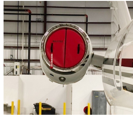
Embraer Legacy 500 Engine Inlet Plugs, folding type
