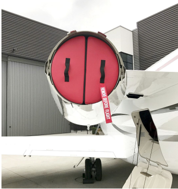
Cessna Citation 680 Exhaust Plugs, folding type
