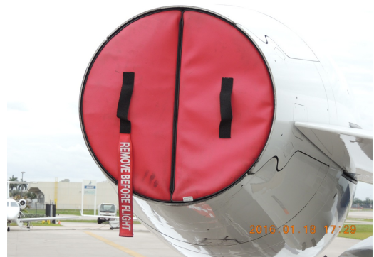
Embraer Legacy 500 Engine Exhaust Plug, folding type
