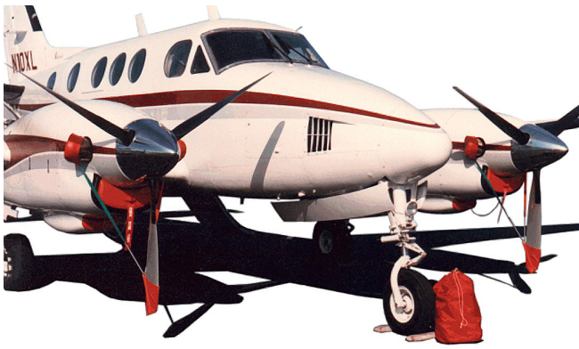
Pitot, Exhaust Covers, Engine Plugs & Prop Ties
