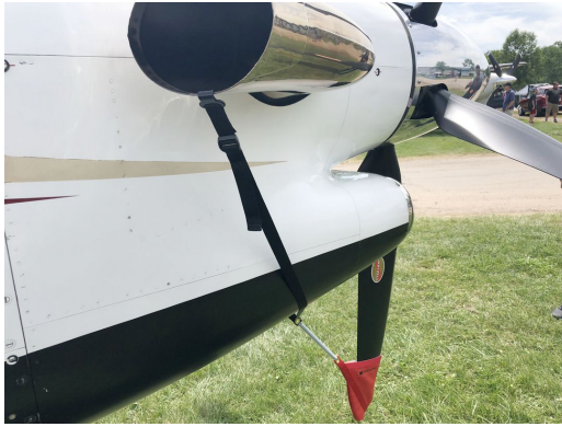
Beech C90A Prop Tie-Down
