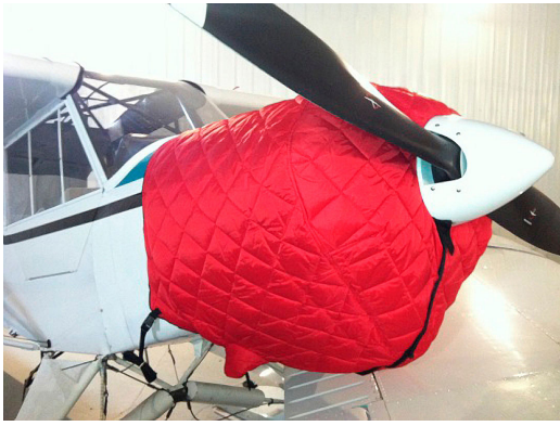
Piper Super Cub Insulated Engine Cover
