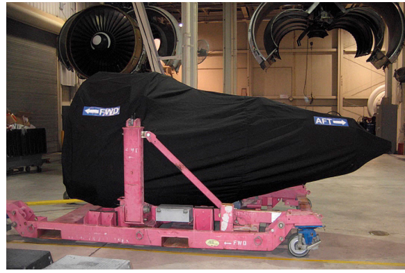
CFM56-5B Off Link Cover, fully enclosed CFM-56-7 Off-link Engine Shipper/Transport cover, w/ Exhaust Cone, fully enclosed
