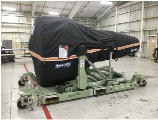
CFM56-5B Off Link Cover, fully enclosed CFM-56-7 Off-link Engine Shipper/Transport cover, w/ Exhaust Cone, fully enclosed
