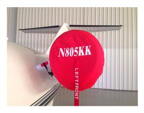
Cessna CJ1 Intake Cover and Inlet Plug
