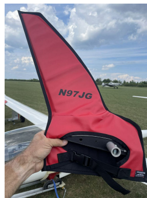
Schempp-Hirth Ventus-2B winglet/wingtip pads
