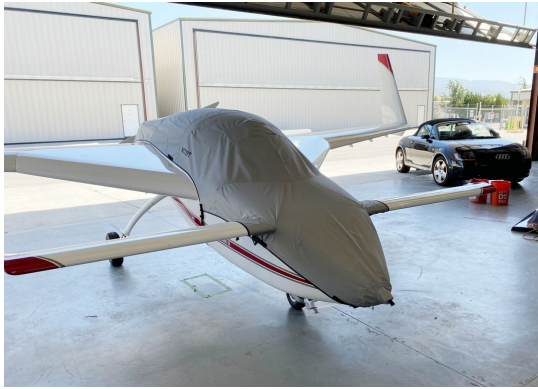
Cozy Mk IV Canopy/Nose/Engine Cover, travel weight design
