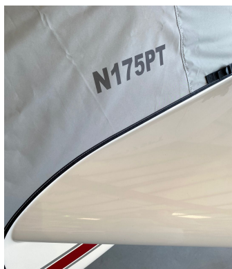
Cozy Mk IV Canopy/Nose/Engine Cover, travel weight design
