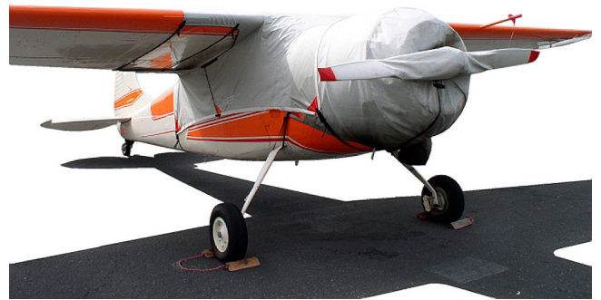
Cessna 195 Over-Top Canopy, Engine & Prop Covers
