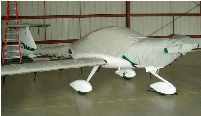
DA-20 Canopy/Engine, Prop/Spinner, Wing, Tailboom, Horiz. Stab. Covers
