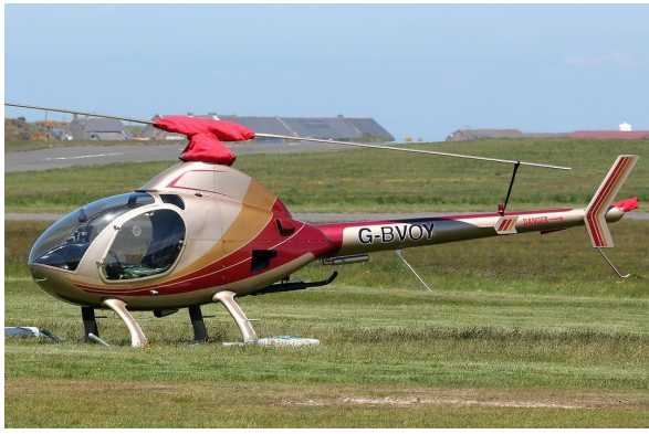
Rotorway Exec 90 Rotor Mast Cover
