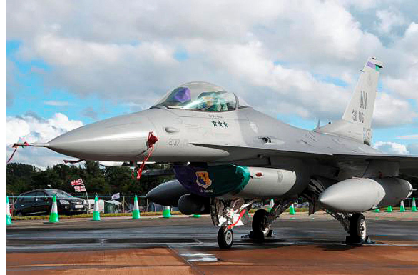
Intake, Maintenance Seat & HUD display covers (Aviano AFB, Italy)
