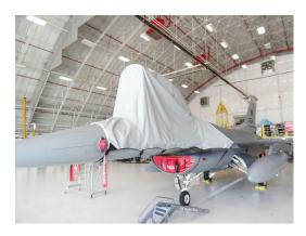
F-16 CANOPY COVER, OPEN POSITION (C-Model, single seat F-16 CANOPY COVER, OPEN POSITION (C-Model, single seat models)
