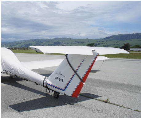
Grob 109 Horizontal Stabilizer Cover
