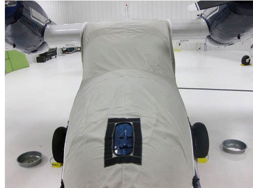
Grumman Widgeon Cockpit/Nose Cover, tie-down cleat detail
