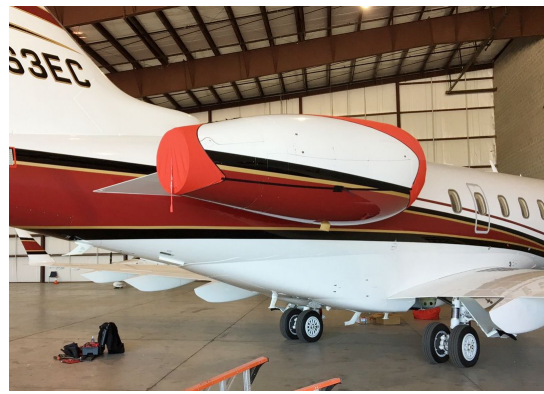
Canadair Challenger 300 Intake/Exhaust Covers, 3-Strap Type
