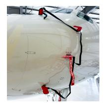
Grumman Gulfstream Exhaust Plugs, folding type
