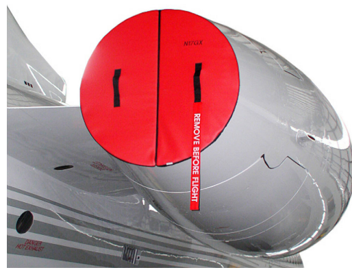
Grumman Gulfstream Exhaust Plugs, folding type
