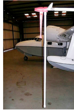
Grumman Mallard Pitot Cover with Install Tool
