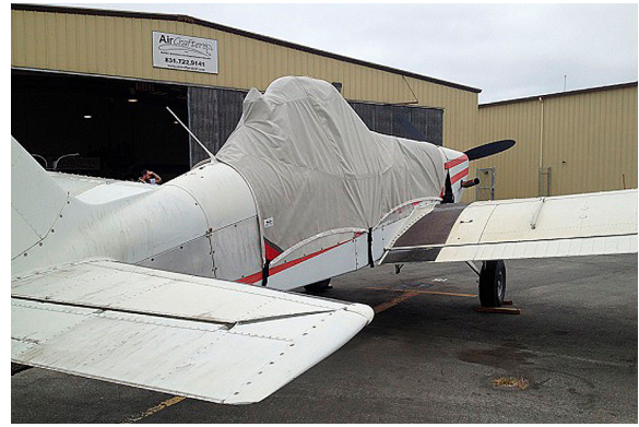
Piper Brave PA-36 Canopy/Hopper Cover
