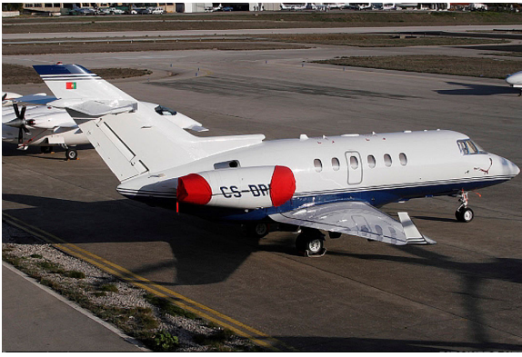
Hawker 900XP Engine Inlet/Exhaust Cover Set & Pitot AOA Cover Set & Cockpit HeatShield Set
