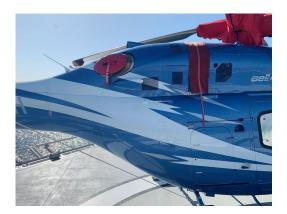
Bell 429 Exhaust Plug, Rotor Mast Cover
