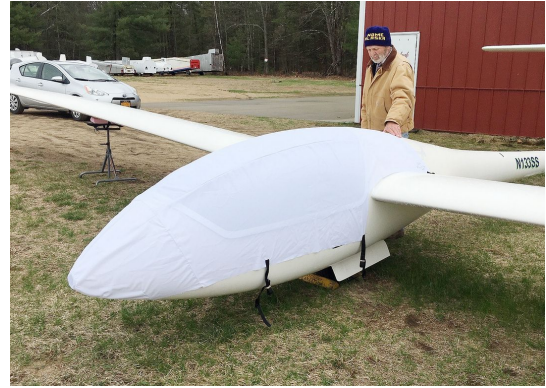
Grob 102 Astir CS Canopy/Nose Cover (test fit)
