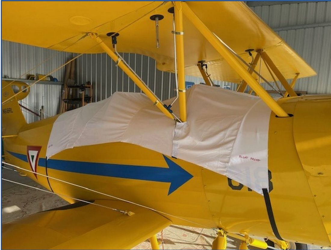
Hatz CB-1 Canopy Cover, test fit
