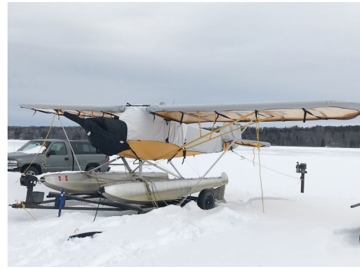
Piper J3 Cub Extended Canopy, Wings, Empennage & Insulated Engine Covers
