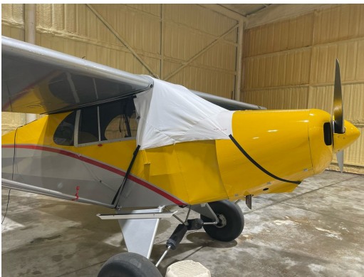
Piper J5A Windshield/Skylight Cover, test fit
