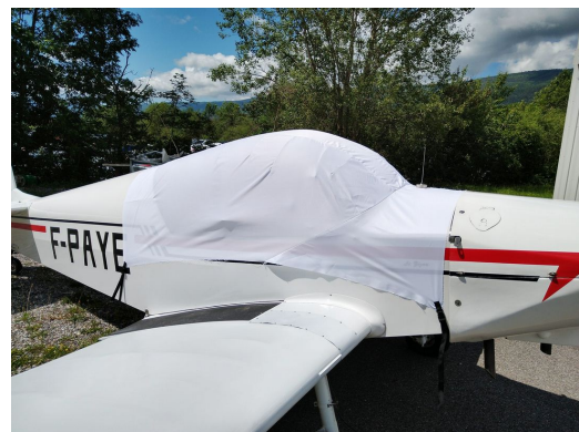
Jodel D113V Canopy Cover, test fit cover
