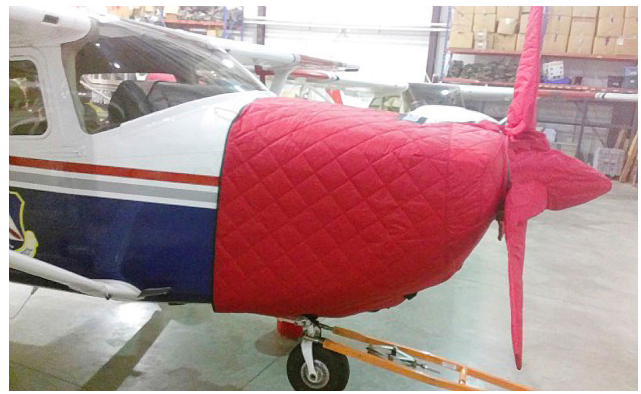
Cessna 182 Insulated Engine & Prop Covers (3-blade)
