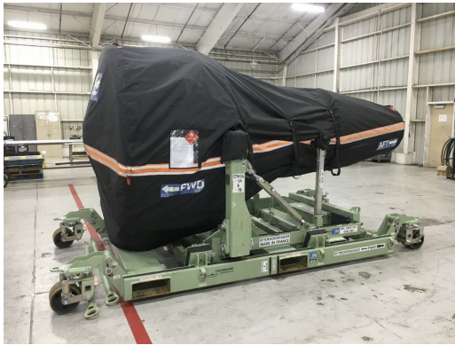
CFM56-5B Off Link Cover, fully enclosed
