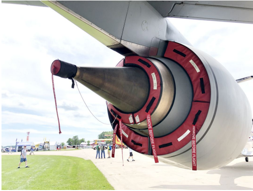
Boeing KC-135 Bypass and Exhaust Plugs
