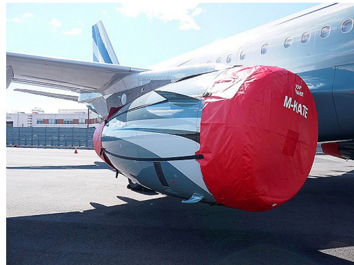
Airbus A319 Intake/Exhaust Covers set, IAE V2500
