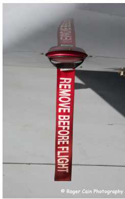
Quest Kodiak Lower Cowling Bypass Duct Plugs
