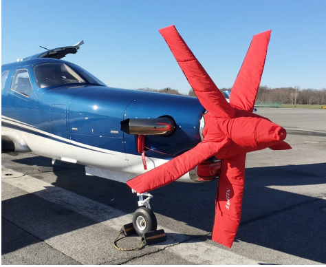
Socata TBM Insulated 5-Blade Prop/Spinner Cover
