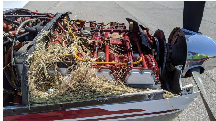
Van's Aircraft RV-7A Engine Inlet Plugs ENGINE PLUGS PREVENT BIRD NEST FOD. Piper Saratoga Engine Cowling Bird's Nest
