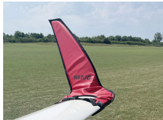
Schempp-Hirth Ventus-2B winglet/wingtip pads
