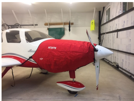
Lancair ES Insulated Engine Cover, Fully Enclosed
