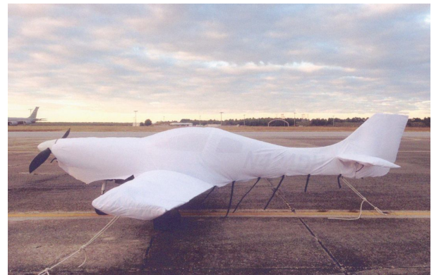
Lancair 360 Full Body Cover, test fit cover
