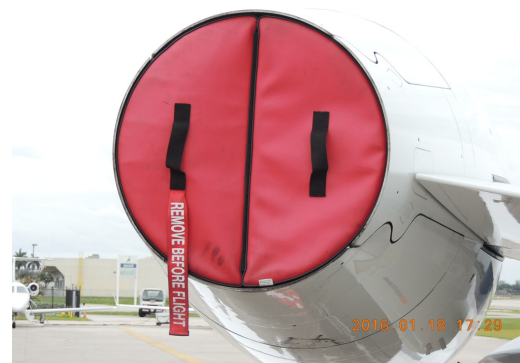
Embraer Legacy 500 Engine Exhaust Plug, folding type
