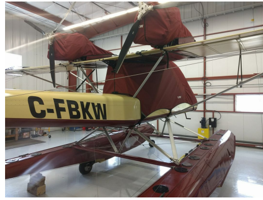
Lockwood Air Cam Canopy Cover, enclosed cockpit style, & Engine Covers
