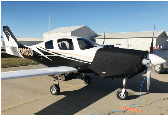
Lancair IV-P Insulated Engine Cover, fully enclosed
