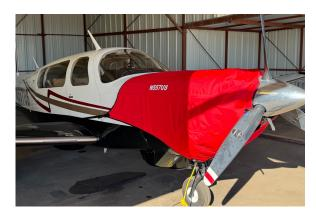
Mooney M20M, Insulated Engine Cover, doesn't cover gear well
