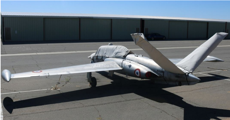
Fouga Magister Canopy/Nose Cover, Tail Stabilizer Covers
