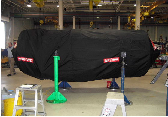
PW JT8D Off-Link Engine Transport Cover (no nose cone, no TR's), fully enclosed
