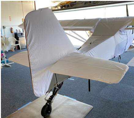
Kitfox Empennage Cover, test fit cover
