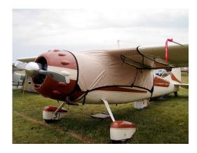
Cessna 195 Canopy Cover, over-top, 24" fwd ext to cover cowl ring gap, Cessna 195 Canopy Cover, extended forward and over gas cap ext.
