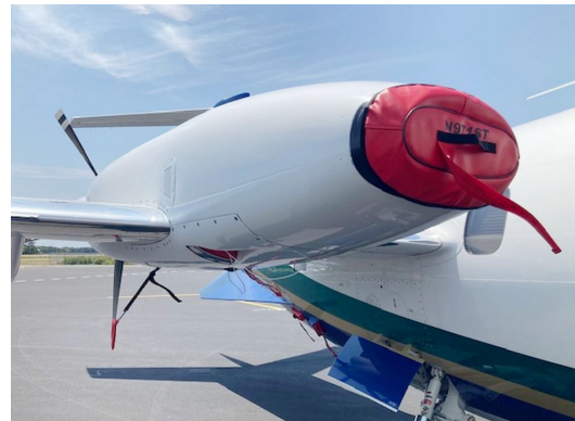
Piaggio P180 Intake Plugs with Fabric Extension
