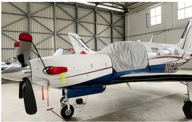
Piper PA-46-500TP Engine Cowling Top Plug
