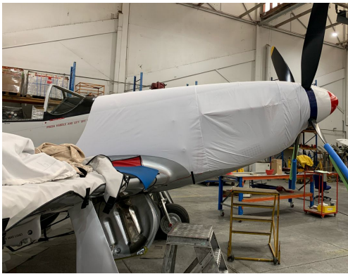
North American P51 Engine Cover, test fit cover North American P-51 Mustang Canopy Cover, Belly Scoop and Chin Scoop Plugs
