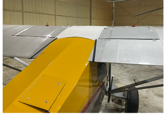
Piper J5A Windshield/Skylight Cover, test fit
