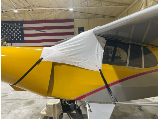
Piper J5A Windshield/Skylight Cover, test fit
