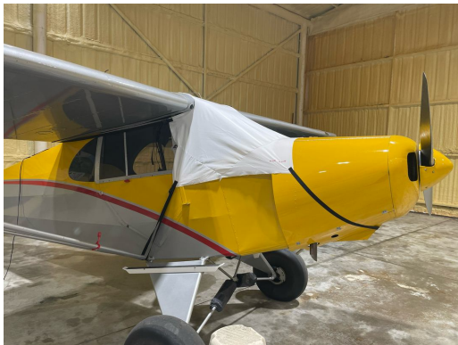
Piper J5A Windshield/Skylight Cover, test fit
