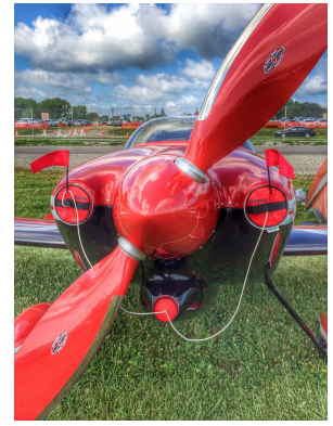
ENGINE PLUGS PREVENT BIRD NEST FOD. Piper Saratoga Engine Cowling Bird's Nest SPA Sport Panther Engine Plugs
