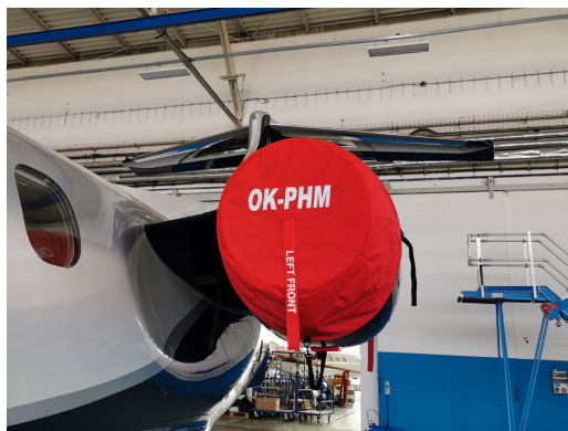
Embraer Phenom 300 ENGINE INLET COVERS & EXHAUST PLUGS (includes lower nacelle plug) (set of 4)
