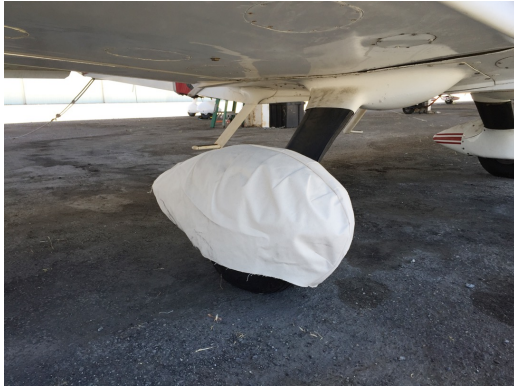
Grumman AA5 Main Wheelpant Cover, test fit
