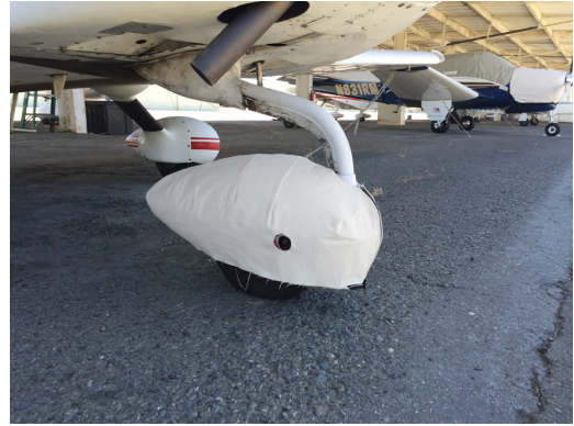
Grumman AA5 Nose Wheelpant Cover, test fit
