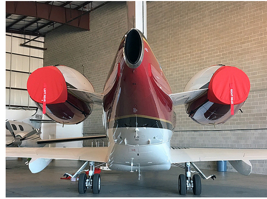
Canadair Challenger 300 Intake/Exhaust Covers, 3-Strap Type
