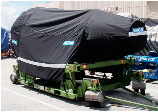
PW 2000 SERIES OFF-LINK ENGINE COVER, "rain cap" style
