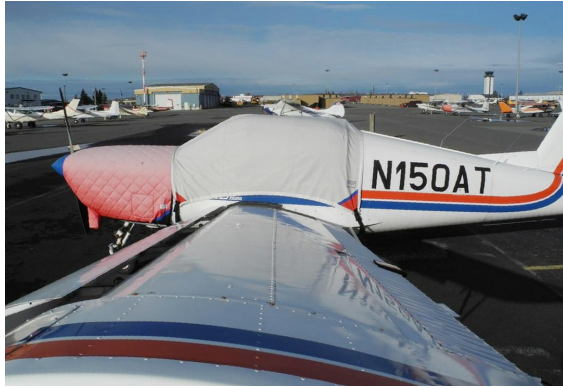
Koliber 150A Canopy Cover, Insulated Engine Cover
